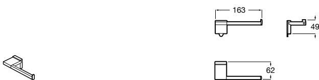
Rubik A816850001 Toilet roll holder without cover (Can be installed with screws or adhesive)
